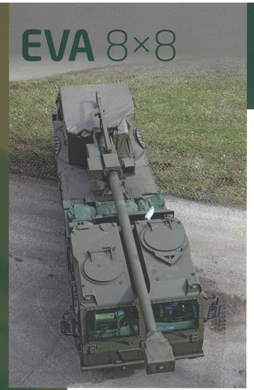
155 mm 52 cal. EVA 8×8 presents a self-propelled autonomous artillery system with automatic loading of ammunition providing an effective fire by means of both direct and indirect aiming. Design is based on a proven 155 mm 52 cal. SpGH while overtaking maximum assemblies and design solutions verified within the course of demanding testing and tender trials performed in Slovak Republic and abroad.
